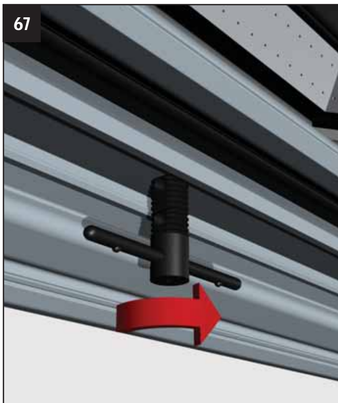
67 Twist through 90° to locate the T bolt into the ridge capping.
