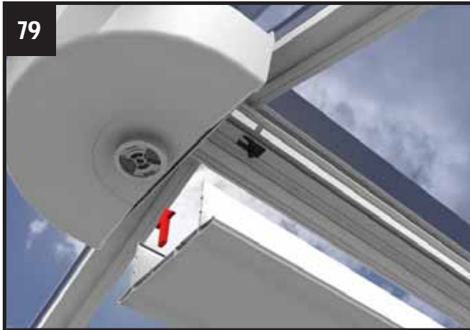
79 Trim to length the main ridge body undercladding and clip in. THIS MUST BE DONE BEFORE INSTALLING THE 'T' SHAPED UNDECLADDINGS.
