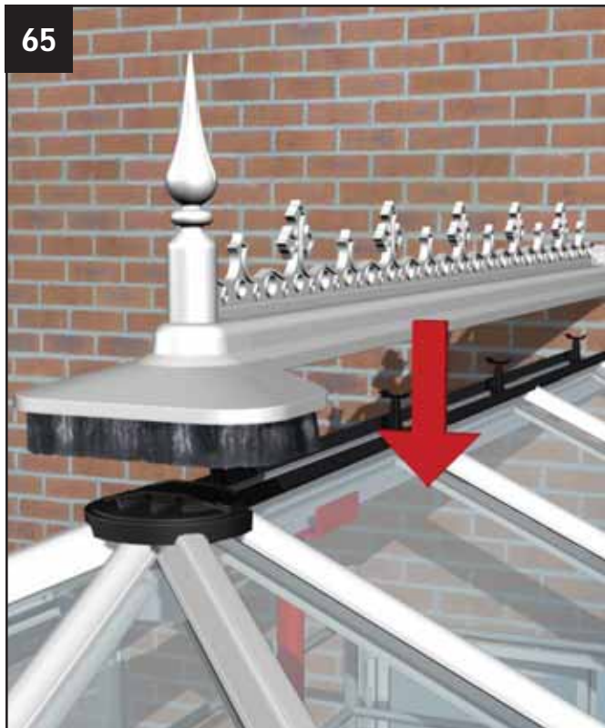
65 Offer up the complete ridge capping onto the roof. Please note. If a Ridgeflow ventilation unit is to be fitted, the air deflector must be attached to the PVCu top cap prior to its fitment. Refer to separate Ridgeflow installation guide.
