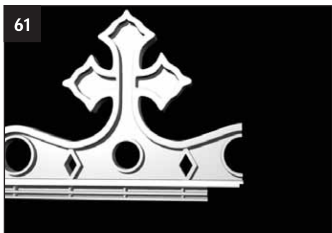
61 Cut back the underside of the last section of cresting by 40mm.
