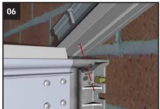
06 Attach the starter bar using the nut, bolt and spring washer (included in the kit) to the eaves structural moulding. Finger tighten the nut to temporarily allow the assembly to hang.
