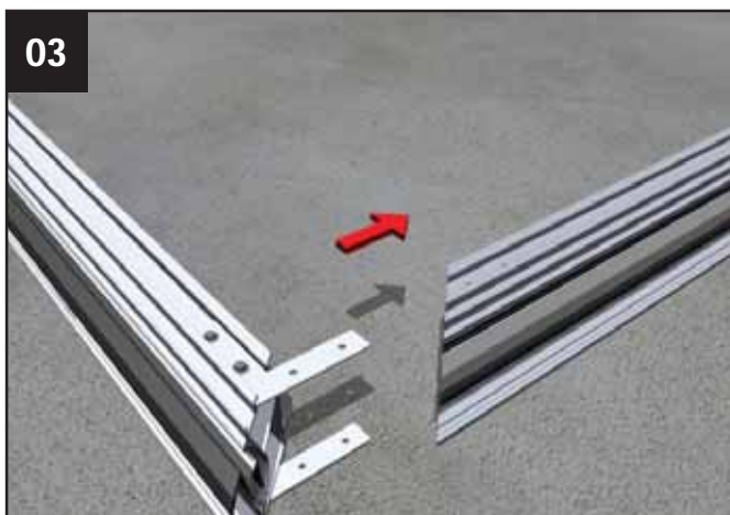
03 Slide the cleated corners into the adjacent piece of lantern beam
