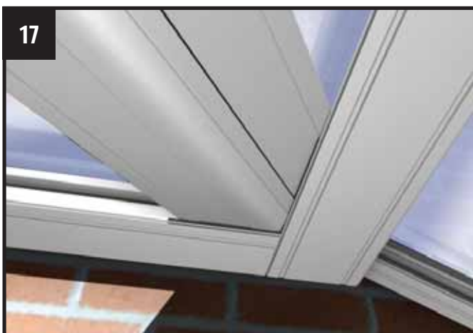
17 Valley claddings shown in situ at the ridge.
